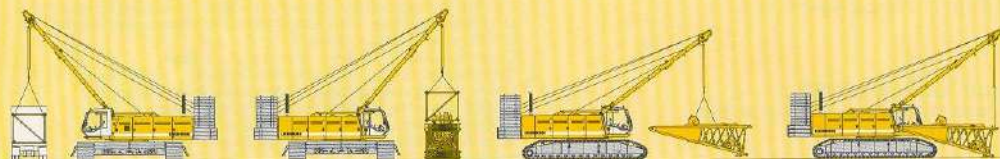
Unloading and assembly of boom - Assembly of boom foot
